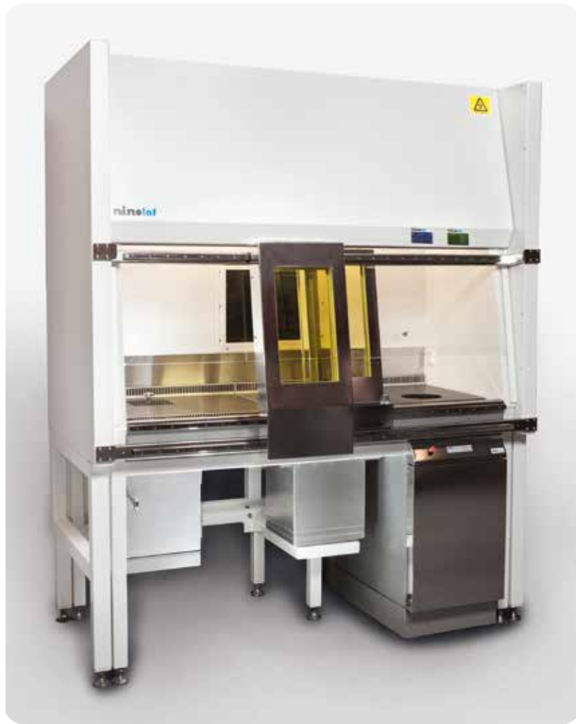
Radiation shielded Microbiological Safety Cabinet combined for both PET and Tc-99 with 50 mm Pb around the cabinet and 30+20 mm Pb equivalent slidable lead glass in front. Integrated generator storage, waste and dose calibrator – all with 50 mm Pb.
